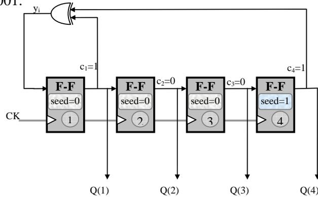
Figure III-2, 4 stage Max-length LFSR
