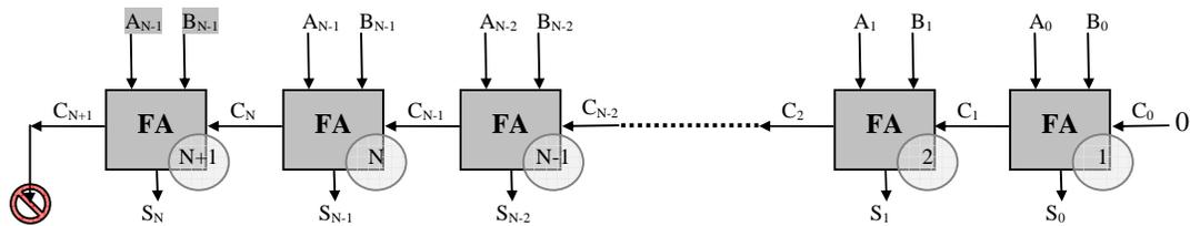
Figure V-3, sign extended addition of signed numbers
