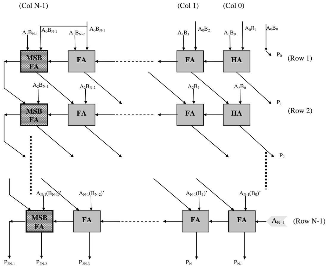
Figure V-15,  $N \times N$  CPA Multiplier Structure
