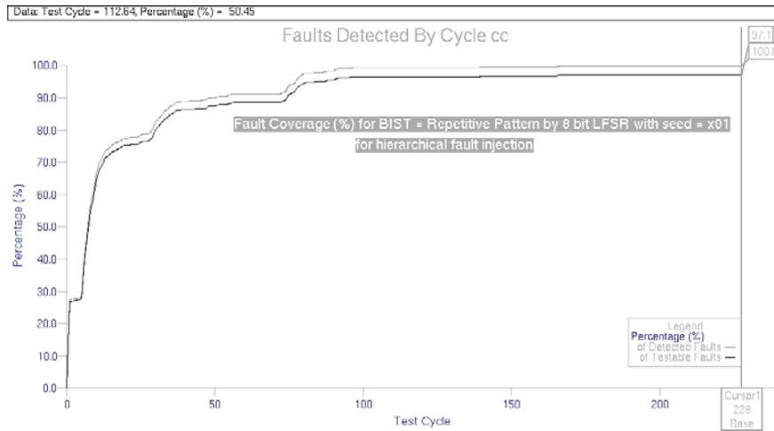
Figure VI-40, Fault coverage (%) for 8 bit LFSR with repetition length,  $k = 4$  and seed= $x01$
