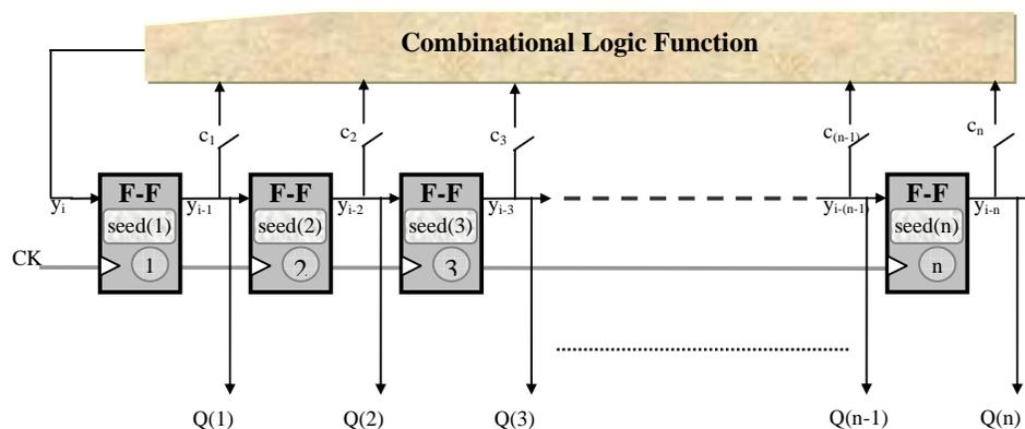
Figure III-4, Nonlinear Feedback shift Register
