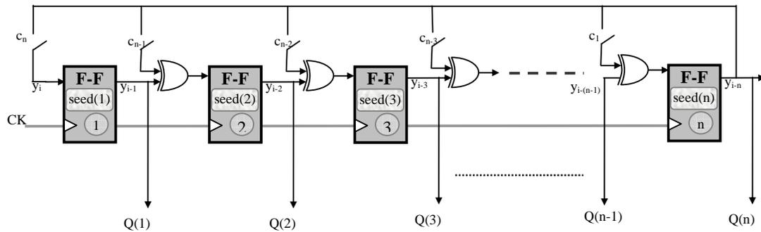
Figure III-3, TDA – LFSR structure
