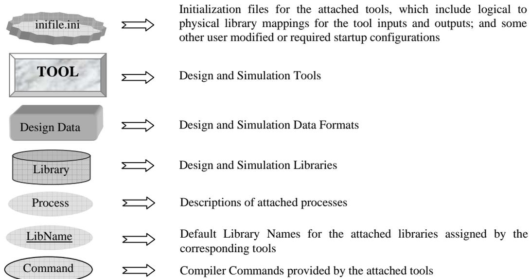
Figure IV-3, Key to Design and Tool flow units
