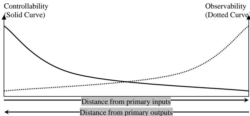
Figure II-1, General Characteristics of Controllability and Observability([13])
