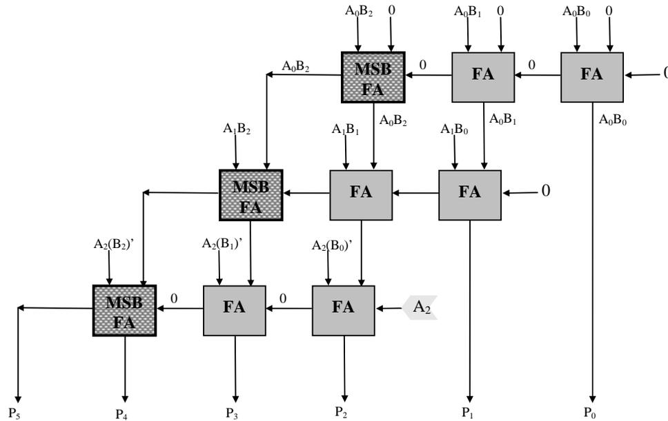
Figure V-5, Regular 3x3 CPA Multiplier Structure
