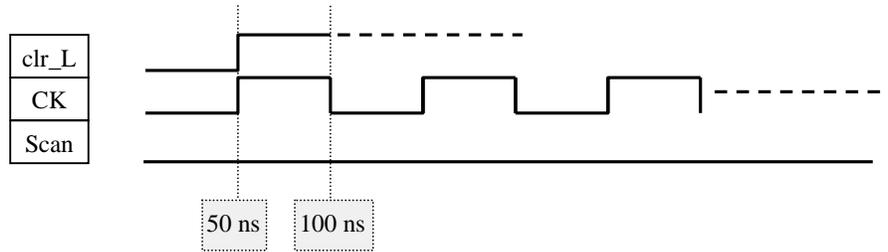
Figure VI-54, Signature analyzer input signals
