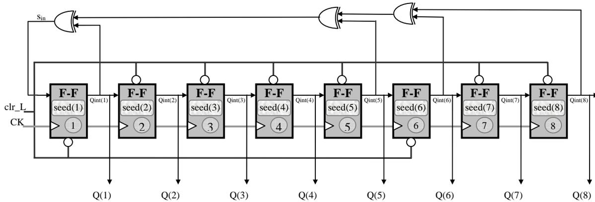
Figure V-21, Structure of LFSR
