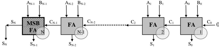
Figure V-4, Modified signed adder
