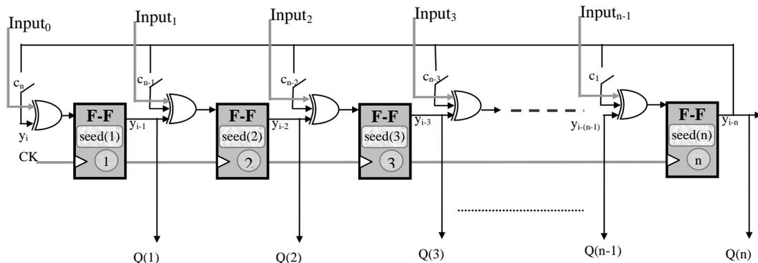
Figure III-7, Multiple Input Signature analyzer
