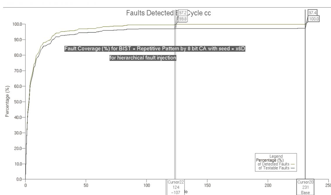
Figure VI-50, Fault coverage (%) for 8 bit CA with seed=x6D
