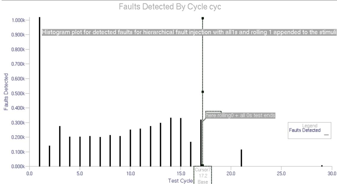
*Figure VI-27, Histogram for rolling0 + all 0s test followed by a rolling1 test*
