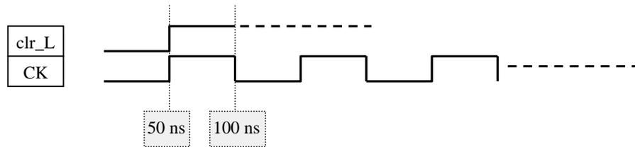
Figure V-22, LFSR Simulation input Signals
