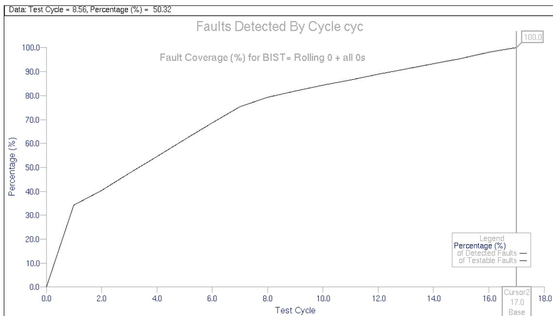
Figure VI-18, Fault coverage (%) for board level rolling0 + all0s test
