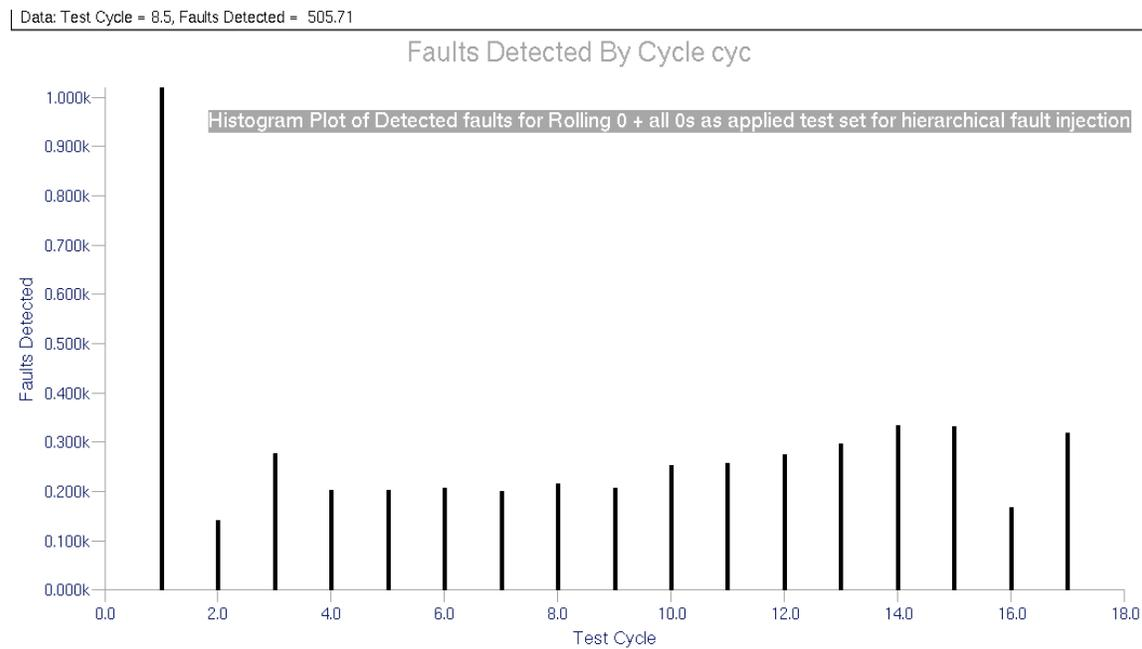
Figure VI-25, Histogram for hierarchical rolling0 + all 0s test
