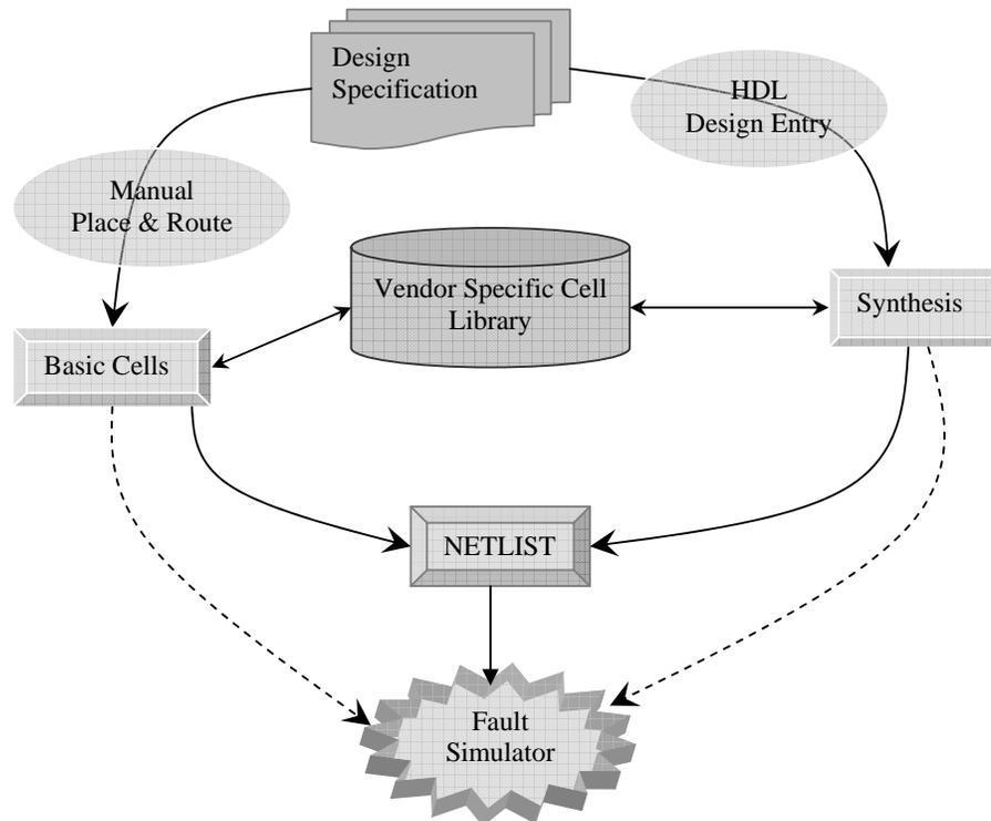
Figure IV-1, Generic Design → Fault Simulation Flow Chart
