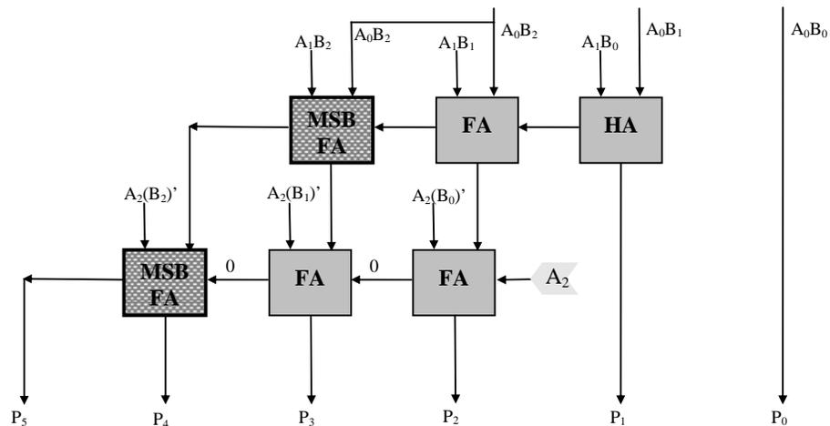
Figure V-6, Used 3x3 CPA Multiplier Structure
