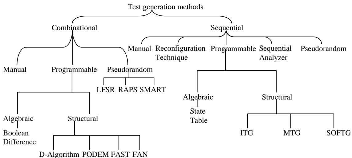
Figure II-2, Test pattern generation techniques ([1])
