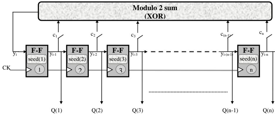
Figure III-1, General Description of the LFSR Structure
