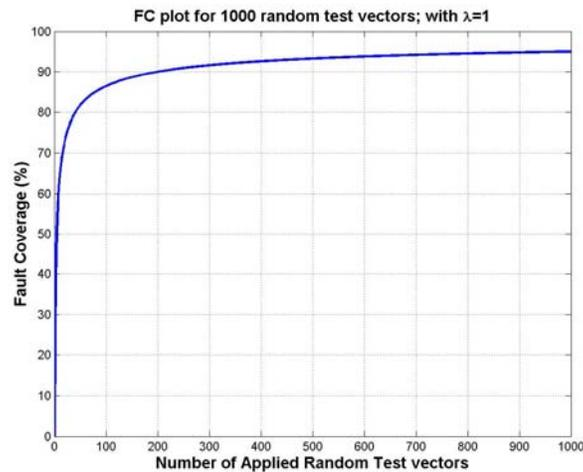
Figure II-3, Fault coverage plot for 1000 random test vectors
