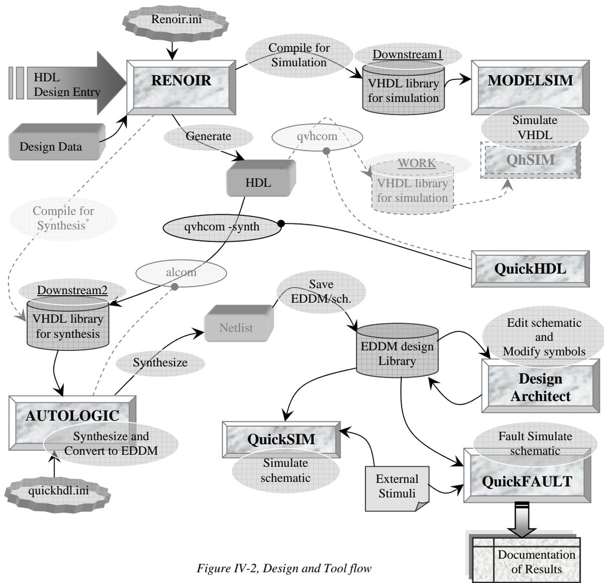
Figure IV-2, Design and Tool flow
