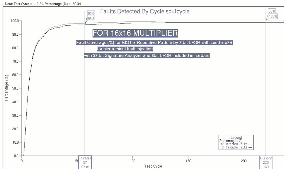
Figure VI-62, Fault coverage (%) for LFSRmultSign16x16
